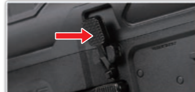
Press the Bolt release lever to release the Bolt catch.
